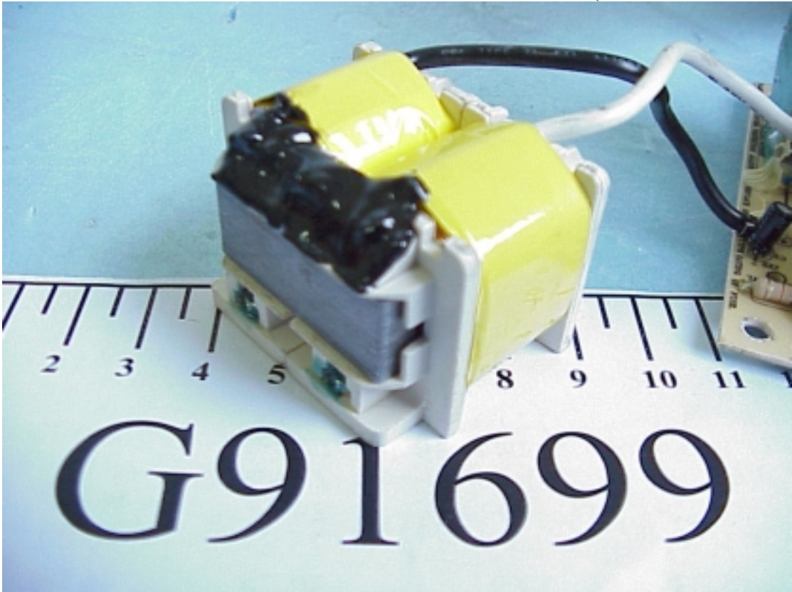
Figure 11 Internal View (PFC Choke/Front View)
