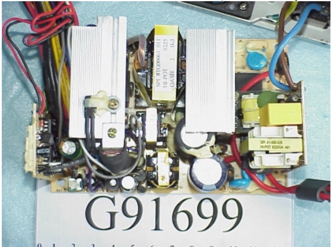
Figure 5 Internal View (Main Board I/Component Side)
