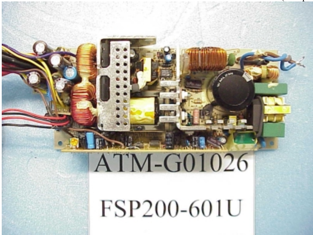
Figure 13 Switching Power Supply, M/N FSP200-601U Main Board (Component Side)
