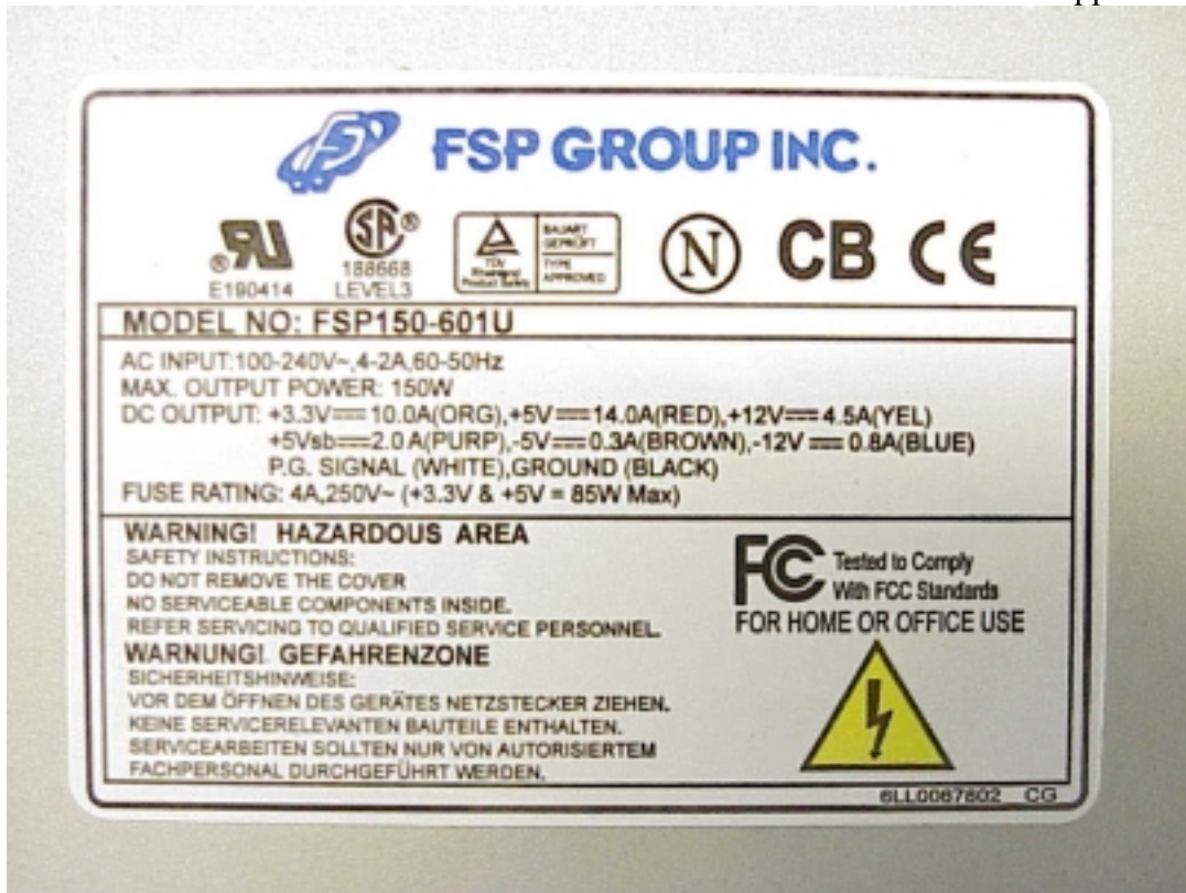
Figure 3 Switching Power Supply, M/N FSP150-601U General Appearance (Label)
