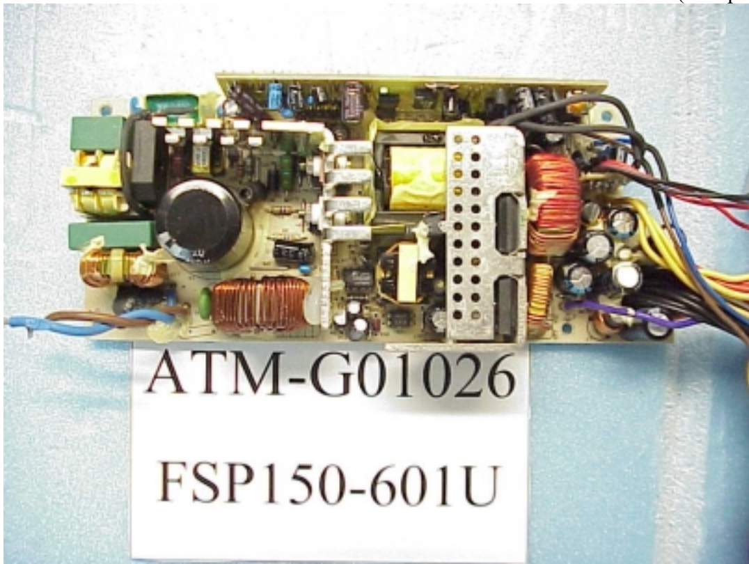
Figure 5 Switching Power Supply, M/N FSP150-601U Main Board (Component Side)
