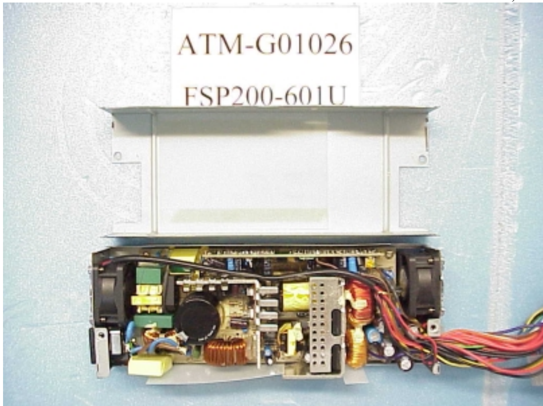
Figure 12 Switching Power Supply, M/N FSP200-601U Cover Removed, Internal View
