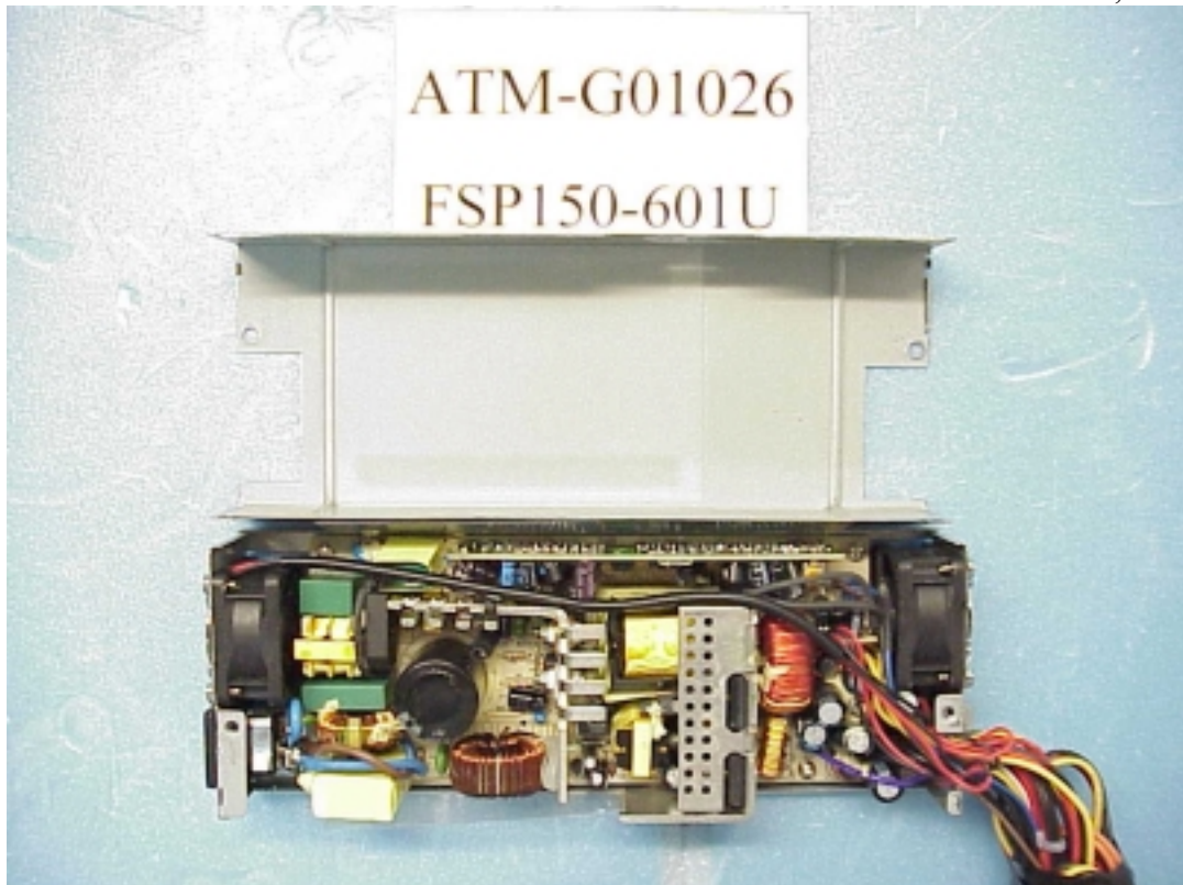
Figure 4 Switching Power Supply, M/N FSP150-601U Cover Removed, Internal View
