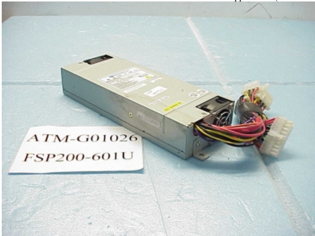
Figure 9 Switching Power Supply, M/N FSP200-601U General Appearance (Front & Side View)
