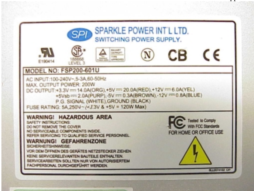
Figure 11 Switching Power Supply, M/N FSP200-601U General Appearance (Label)
